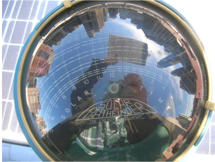
Figure 2-14: Solar Pathfinder On-Site Close-Up – on top of Friends Center, Arch St., Philadelphia (objects shading the site are reflected in dome of device)
